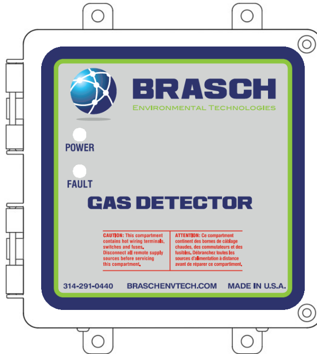
Figure 9: Transmitter Front Cover Layout
