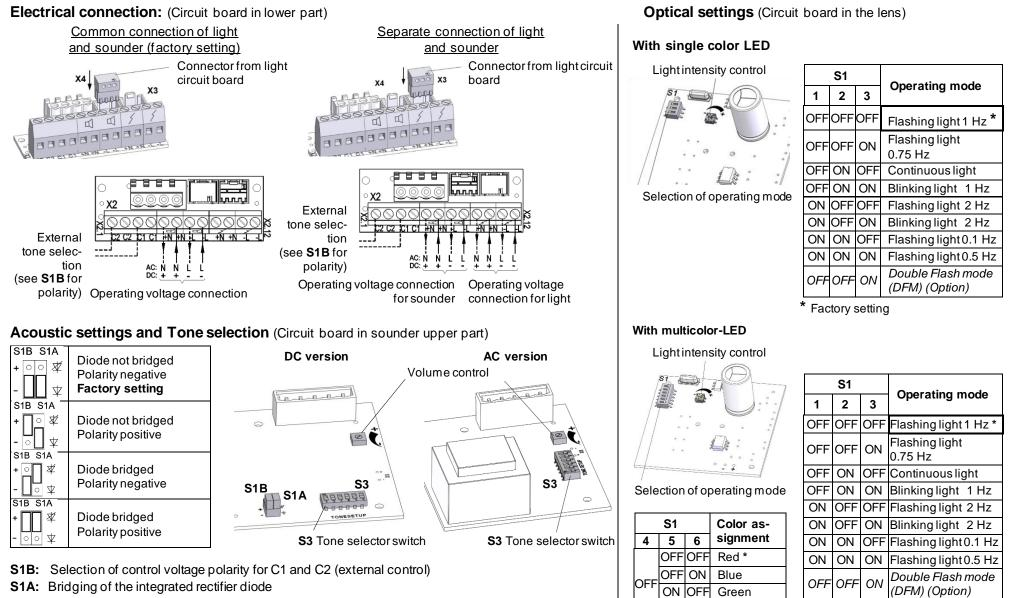
The desired tone can be selected using the **S3** tone selector switch. The tone is generated after the supply voltage is applied. A complete tone type table can be found in the Annex. See the digital operating instructions for the external control of other tones, source: <u>www.pfannenberg.com/manuals</u>
